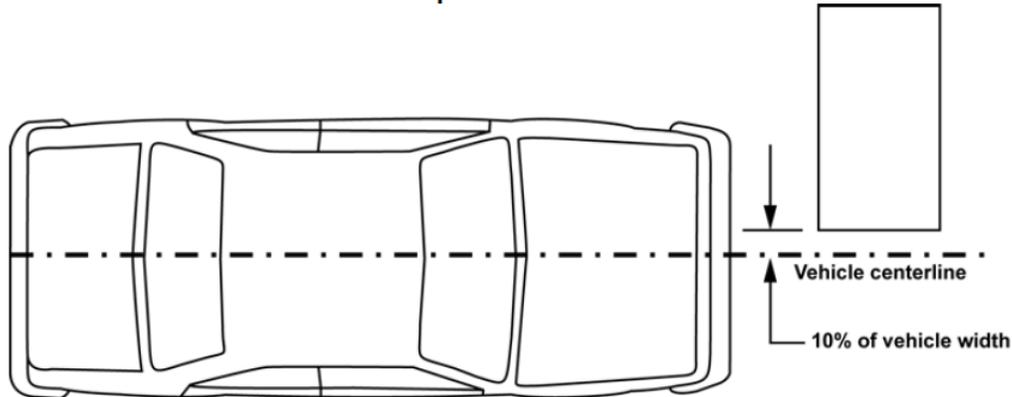
A total of 14 measurement locations are used in general (on the driver-side interior & exterior of the vehicle) and their longitudinal, lateral & vertical displacements with respect to a user defined coordinate system are measured.
