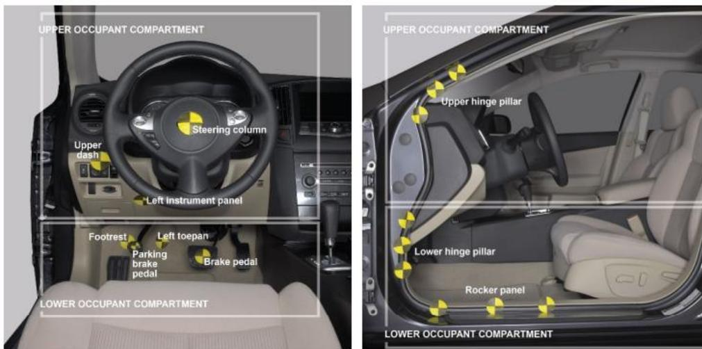
Locations for Measuring Vehicle Intrusion – Passenger side:
