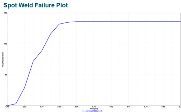
1D beam spot weld / Single hexa spot weld report
