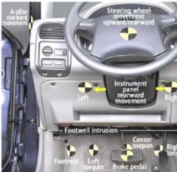
Steering column (one point), lower instrument panel (two points), brake pedal (one point), toepan (three points), left footrest (one point), seat bolts (typically four points, each of the 4 bolts that anchor the driver seat to the vehicle floor), A-pillar (one point) and B-pillar (one point marked at the same vertical coordinate as the lower A-pillar mark).
