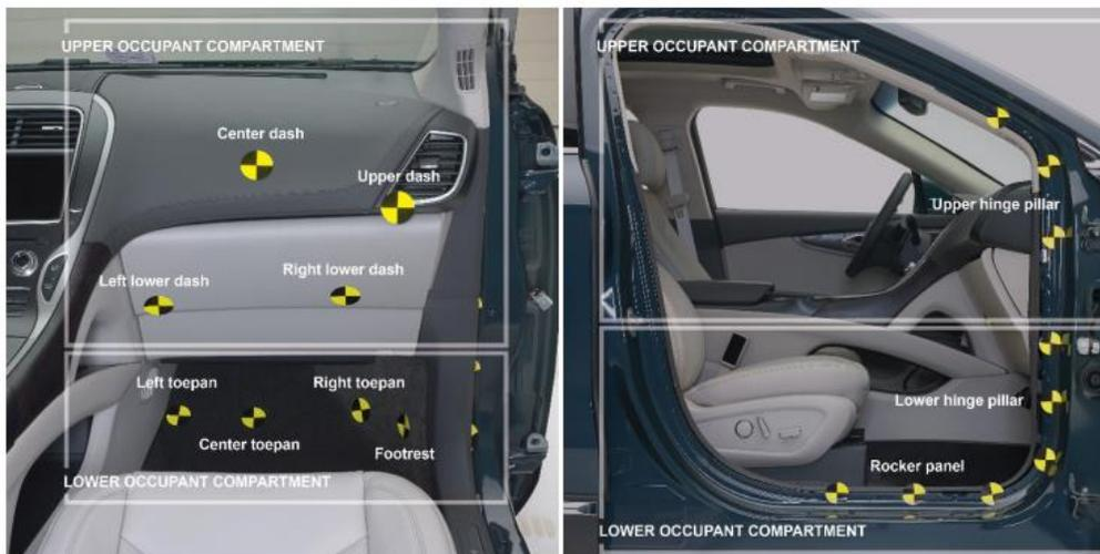
Steering column (one point), left instrument panel (one point), brake pedal (one point), parking brake pedal (one point), footrest (one point), seat bolts (two points), left toe pan (one point), upper dash (one point), lower hinge pillar (three points), upper hinge pillar (three points) and rocker panel (three points).
