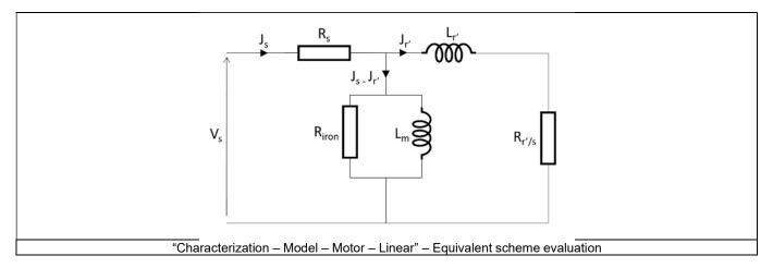
The resulting equivalent scheme corresponds to the original model or the refined one according to whether a refinement has been performed or not.
