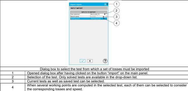
Note: The imported data are the output data directly shown in the considered solved test. For some tests, some values are not defined (like for instance the rotor iron losses or the Mechanical losses). In that case, the corresponding input in transient thermal test will remain at the value existing before the import.
