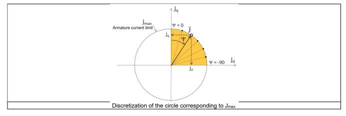
Then an optimization process is performed to get the base speed point which corresponds to the working point at maximum line current and maximum line-line voltage:  $I = I_{max.}$  and  $U = U_{max.}$ .
