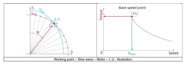
The results of this test give an overview of the electromagnetic analysis of the motor considering the machine topology. The general data of the machine, like machine constants and the power balance are computed and displayed. The magnetic flux density is also computed in every region of the machine's magnetic circuit to evaluate the design. In addition, ripple torque at the base speed point is computed.
