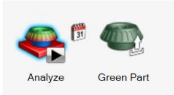
After a compensation analysis, Inspire Print3D can compute the Green Part that needs to be printed in order to produce the desired shape after sintering.
