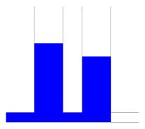
The control consists of turning on and off a pump, which can inject liquid in the first tank with a constant flow. The second tank is emptied through a valve, placed at the bottom of the tak, which is opened and closed at random times. The pipe connecting the two tanks is also placed at the bottom of the tanks.
