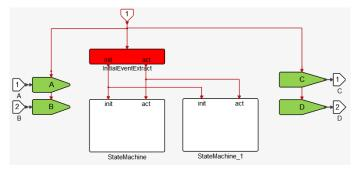
Two parallel running state machines, and two inputs and outputs are assumed in this skeleton. The content is specialized to this case as follows
