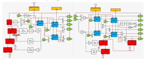
The **ActivatedIntegral** blocks are used to implement the differential equations of the system and their (re-)initializations.
