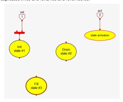
To implement the transitions and the actions, note that in the Statechart model the entry actions are placed inside the states and the transition conditions on the outside. In **Twin Activate** both are placed inside the **StateBlock** blocks. Starting with the first state, Init, the skeleton
