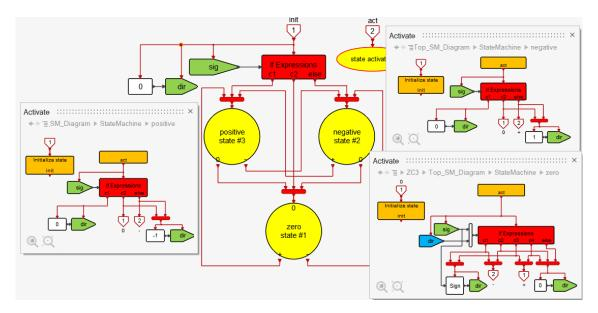
The 3 states of the state machine correspond to the sign of the latest input. The main logic of the detection is implemented by the **IfExpressions** block in the zero state block, parameterized as follows
