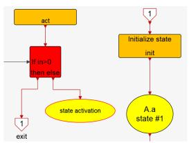
The substate A.a is initially activated every time the state A is entered. Other initialization actions can also take place by init. The act signal activates actions during the activity of state A. In this example, these actions activate the state machine inside A, and when some condition is satisfied, causes an exit from A.
