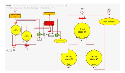
The contents of the states implement the system equations in different situations. Note that  $A_1$  can may exit before any activation of the substates  $B_1$  and  $B_2$ . This happens if the magnitude of  $\dot{\theta}$  is above a threshold. In this cases the block bounces back instead of lying flat.
