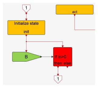
It may seem interesting to leave a state right-away at initialization when a condition is true, even before activating the state. But this could lead to unexpected behavior. The next state will be initialized synchronously with this state, so not only the initialization actions may be in conflict, but even the setting of the state is in conflict, so there is no guarantee as to which state becomes active following the double initialization.
