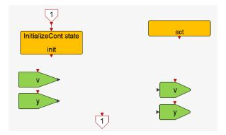
The **InitializeCont** block is the continuous-time counterpart of the **Initialize** block. The **Action** and the set and get blocks are the same as in the discrete-time case.
