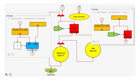
The process time here is assumed constant equal to 1. Other models for the process time can be implemented by simply using other inputs to the timer block instead of a constant. The process time can be made random, deterministic but time varying, or even made dependent on the model states, for example on the number of clients waiting in line.<sup>1</sup>
