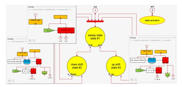
The shift up and down events changes the gear signal in the parallel state machine
