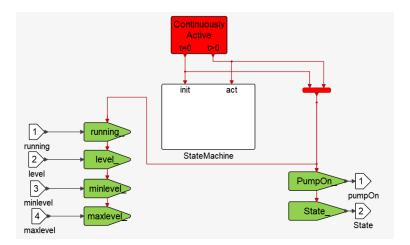
The state machine uses 3 states, as in the discrete-time implementation:
