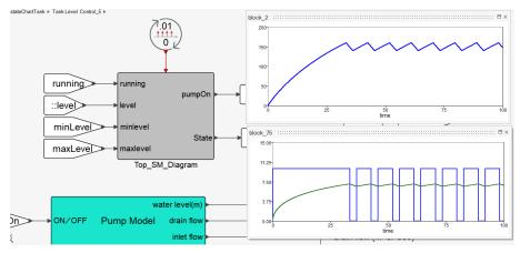
The block-based construction of state machines in **Twin Activate** seems to require more work than the use of specialized state machine modeling paradigms. However, the construction is carried out fully in "native" **Twin Activate**. A single language (**Twin Activate**) is used in the construction of the complete
