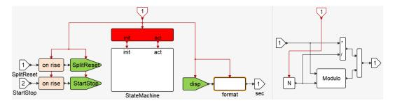
The StartStop and SplitReset signals become true when the corresponding buttons are pressed. The disp signal contains the time to display in seconds. The format super block (content shown on the right) converts the value of time to two values: number of seconds and hundredths (or tenths depending on the value N) of seconds.
