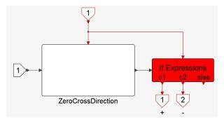
Note that the zero-crossing detection generates events that are synchronous with the input signal. There is no delay in detecting the crossings.
