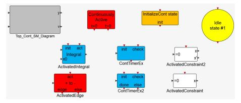
Some of the blocks replace similar blocks used for the construction of models in the discrete-time case. Others are specific to the usage in the continuous-time, for example the constraint blocks and zero-crossing blocks.
