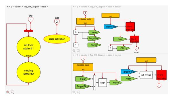
Entering in the atFloor state, the move (elevator motor command) and TargetFloor signals are set to zero, and the elevator door opening is initiated. Then the TargetFloor is monitored; if it becomes non-zero, then the door is checked. If closed, the state changes, if not the closing is initiated, and the checking repeated.
