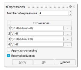
Using the C code generation option in the Tools menu, the **Top\_SM\_Diagram** can be converted into a CCustomBlock, and then turned into a basic block. This block can be used for example to build an alternative to the Activate **EdgeTrigger** block as follows
