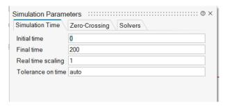
This value is set by default to 0, corresponding to no slowdown of the simulation. Non-zero values set the ratio between the simulation time and the real time; the value of 1 indicates one second per unit of simulation time. The larger this value, the more the simulation is slowed down.
