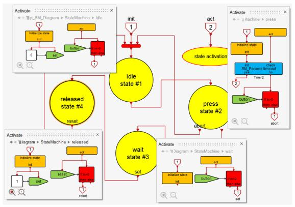
Note that the timeout parameter is used in the Timer2 block as SM\_Params.timeout, defined in the context of the Top\_SM\_Diagram super block:
