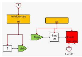
Its operation is straightforward to understand: the state signal is initially set to 2, and subsequently the temperature is tested, leading to an exit if it goes beyond 25.
