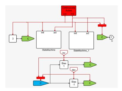
An extended state (signal C) is used to hold the state of the queue, i.e., the number of people waiting. This state is incremented and decremented by the transitions within the two state machines. The incrementing is done by the arrival event, generated by the first state machine shown below
