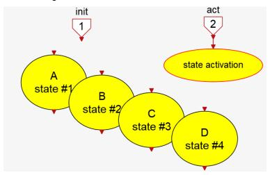
A unique number is associated with each **StateBlock**, and the **StateActivation** block redirects its activation to one and only one of these **StateBlock** blocks at any time. The **StateActivation** block is
