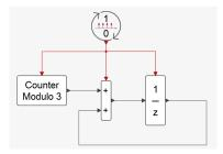
the Counter, the Sum and the Delay blocks are activated synchronously every unit of time<sup>2</sup>. The state of this system/model is constituted of the internal states of the blocks, in particular the internal states of the Counter and the Delay blocks. The model state is not apparent on the diagram but hidden inside its individual constituents.
