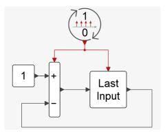
In this case there is no algebraic loop present in the model. The corresponding equation is  $X(t_k) = 1 - X(t_{k-1})$ . The LastInput block introduces a one-step delay in the loop, thus breaking it.
