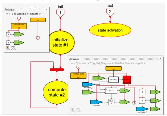
The first state initializes the counter I and the partial sum S, the second state performs one iteration for each action. But the state 2 loops back and re-initializes itself. Even though no action is defined for this re-initialization, with the run-to-completion option true, act is activated immediately, again resulting a
