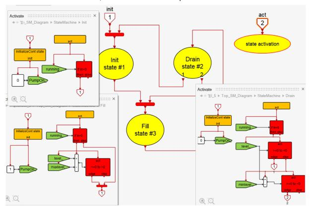
In this implementation the inequality tests in the original StateCharts model are implemented with zero-crossing tests. The **ActivatedEdge** blocks are used to detect the crossings of the threshold temperatures. The simulation can now be performed using variable step-size solvers.
