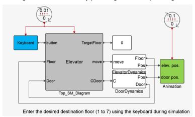
The simulation result is illustrated via a simple animation showing the movements of the elevator and its door.
