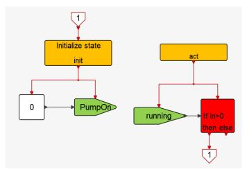
Note that both the Entry action and the exit condition are captured inside the state. **StateBlock** for state 2 is specialized as follows
