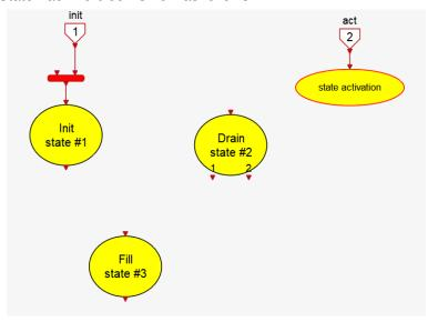
and transitions can be realized by connection the state block ports. A block to obtain the current state number is also used to provide this information as an output (used in the original diagram to display the current state):
