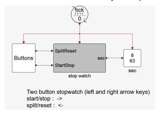
The standard operation of the stopwatch consists in using the start/stop button to start the stopwatch and then stop it. The split/reset button then resets the time to zero. If the start/stop button is applied again instead of the split/reset, the stopwatch restarts from the time it was stopped at. Its subsequent application stops the time again. This start-stop operation can be repeated indefinitely.
