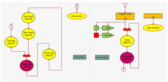
In most cases the simulation is too fast for the animation to be visible. To reduce the simulation speed, the Setup menu for Simulation Parameters can be used to set a non-zero value for the Real time scaling parameter
