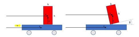
On the left figure, the block is flat on its base and moves along with the cart or slides on the cart surface, due to friction between the base of the block and the surface of the cart.
