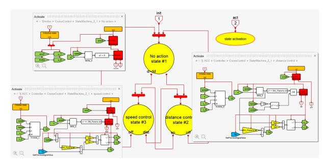
When the ACC is active, the state machine can either be in the speed control state or the distance control state. Each controller is implemented by a PID. The states of the PIDs are initialized when the corresponding state is entered to guarantee smooth transitions.
