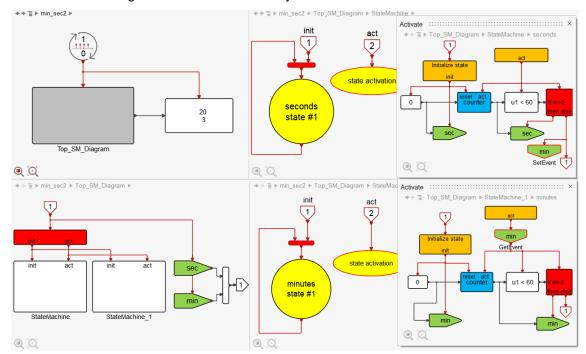
This model functions correctly if the run to completion option is set to false. For models relying on state activations to correspond exactly to source activations, setting this option to true may have unexpected results: the simulation result could be incorrect or the simulation may hang in an infinite loop at a time instant.
