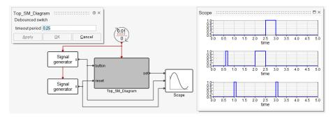
In this case timeout=0.25, so the first button press, which lasts less than 0.25 seconds, does not set the switch. The second press does it once the button is released. The switch remains set until it is reset by the reset signal.
