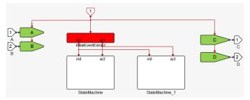
By default, two parallel state machines are assumed. Two inputs and outputs are also named for use inside the state machines. StateMachines are plain super blocks but contain state machine prototype blocks (to be adapted to the application).
