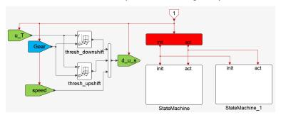
The gears are shifted based on thresholds provided by lookup tables; they depending on the vehicle speed and the throttle position. The decision to shift up or down however is not applied immediately. They are realized only after a period of time if the threshold crossing remains valid. If the threshold is crossed back during this period, the shift is abandoned:
