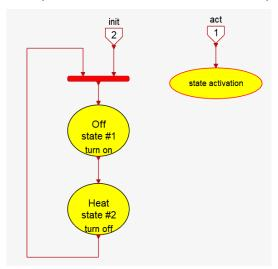
Using the library blocks, user needs not worry about the implementation of the state update mechanism. He/she creates the diagram by placing the state blocks and a state activation block in the diagram (state blocks must be given unique numbers; this constraint is not imposed at construction time, but it is verified by the compiler). The contents of the block states implement their actions.
