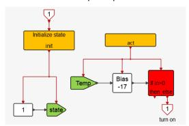
The **Initialize** block receives the event entering the state block, i.e., the event associated with the transition to this block. The initialization event here is used to set the value of the output signal state to 1. After initialization, the act block provides activation signals, which are used to test if the input temperature (Temp signal) has fallen below 17, in which case the event exits the block, initializing the Heat state. The content of the Heat state is shown below
