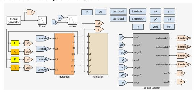
The model represents the dynamics of a 2-wheel vehicle moving straight (no steering) on a non-flat surface. The wheels can be in contact with the ground or be off the ground. So, each wheel can be in two different states (on or off the ground). Only parts of the continuous-time dynamics of the overall system depends on these states, so part of the dynamical system is modeled outside of the state machines, and part of it, inside.
