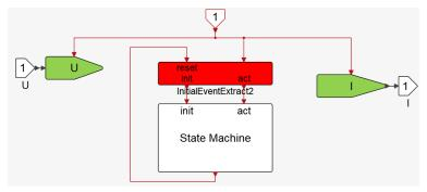
In this construction, each outside activation yields first an init event followed by act event due to the run to completion option. The **InitialEventExtract2** block has a reset port, which once activated, restores the initial behavior of the block, i.e., the next event is directed to the init port.
