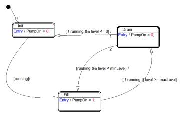
This system has clearly 3 states and the top left state is the initial state. The PumpOn value is set to 0 or 1 when entering different states, and the transition conditions are visible on the arcs connecting them. The content of the StateMachine block can now be specialized to this case. Originally it contains
