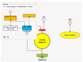
The model uses a single state, which implements a random delay before transitioning. Note the use of the **ContTimerEx** block which generates an event at the end of a time-out period. The time-out value is provided by the input signal at block initialization. So, in this case, the time-out period is a random number.
