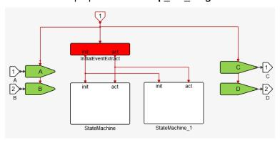
At the top level, it is recommended to use this additional level of hierarchy even if only one state machine is present. This creates a separation between the management of inputs and outputs inside the block **Top\_SM\_Diagram** and the state machine itself.
