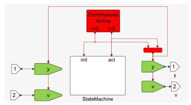
The **ContActivation** (Continuously Active) block provides an always active activation signal similar to the activation signal provided by the **AlwaysActive** block but separated in two: the initial activation signal and the rest of the activation signals.
