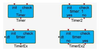
They all work on the same principle: an event on the init activation port starts the timer. An event on its check activation port is then directed to the output if the specified time-period, called timeout, is over. So, the event on the check port "checks" if the timeout period has run out or not.
