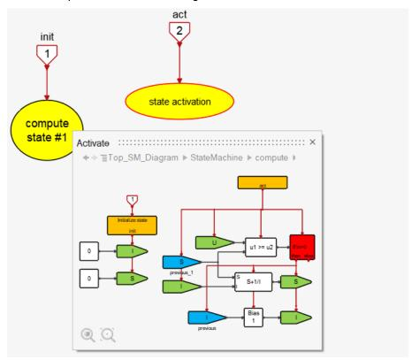
The simulation result shows that the value of I is computed but takes multiple time steps to reach the correct value as it can be seen below. This is not a satisfactory implementation since even if an initial delay at the start to reach the correct value of I is acceptable, if the input is not constant, the output may never be correct. The reason is that the signals I and S are not reset when the input changes.
