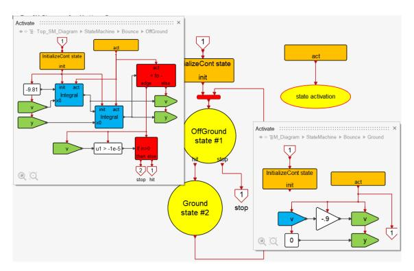
In the OffGround state, **ActivatedIntegral** blocks are used to solve for the speed v and position y. The contact with the ground is detected by an **ActivatedEdge** block. This block generates an event at contact causing an exit from the state. Two possible exits are possible depending on whether the speed of the ball at contact is below a threshold or not.
