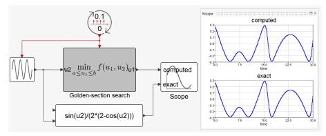
The same block can of course be implemented as an **OmlCustomBlock**, or a **CCustomBlock** for more efficiency. The state machine implementation is converted to C code (thanks to Atomic property of the **Top\_SM\_Diagram**), so the performance is higher than an OML implementation but does not reach that of a well written C code used within a **CCustomBlock**.
