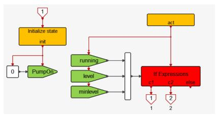
But in this construction, the expressions are not seen on the diagram, so the diagram is less readable, at least for the purpose of the presentation in this document. Note however that the **IfExpressions** block is very convenient to use for defining exit conditions. It is a super block containing a cascade of **IfThenElse** blocks associated with logical expressions.
