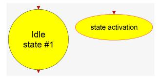
These two blocks go together. They are the basic components for defining a state machine, which is obtained by placing one **StateActivation**, and one or more **StateBlock** blocks in the same diagram. The **StateActivation** block dispatches its activation to one of the **StateBlock** blocks defined by the value of a hidden state variable. The value of this variable is set inside the states, when the states are initialized.
