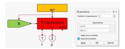
Note also that the use of the cascaded construction is particularly useful for implementing priorities when multiple exit conditions can be true simultaneously.
