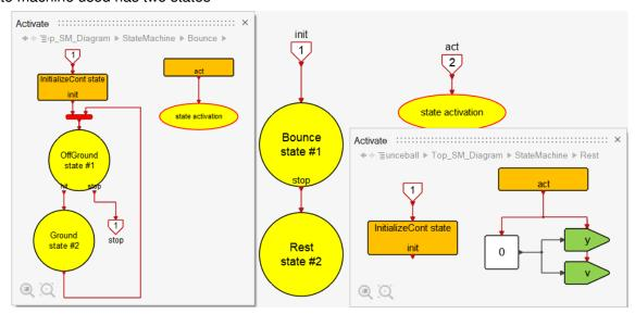
one representing the bouncing state, and the other the resting state. The system can transition from the bounce state to the rest state, but not the other way around. The bounce state contains another state machine corresponding the case where the ball is in the air, and the case when the ball hits the ground:
