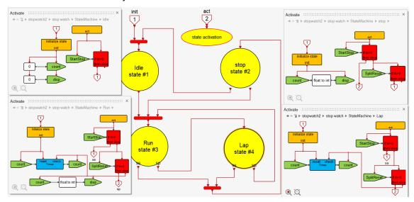
The "float to integer" super block converts the count signal, which has data type double representing the number of seconds, to an integer after multiplying it by N, to be used for display. The operations of different states are clear from their contents.
