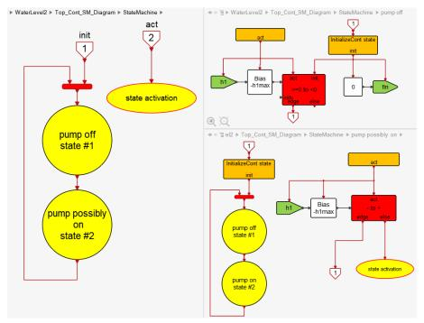
switch between two states: pump off, and pump possibly on. In the second state, the pump can be on and off depending on the level h2. This is modeled using another state machine with two states
