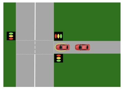
This model contains 5 states representing each a combination of the color of the traffic light on the main road and that of the secondary road: Red|Green, Red|Yellow, Green|Red, Yellow|Red; a transient Red|Red state is also considered for when the traffic light is turned on.
