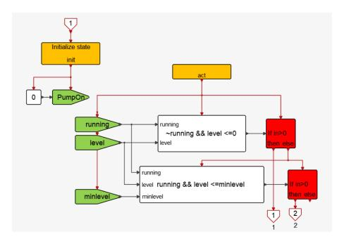
The order in which the **IfThenElse** blocks are placed gives priority to the first exit to be consistent with the arc numberings in the original Statechart diagram. These conditions can be implemented in a simpler way using a single **IfExpressions** block:
