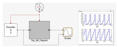
Note that in this diagram, the repeated operations taking place inside the **Top\_SM\_Diagram** are transparent; the block at each activation provides only one output corresponding to the result obtained at the final iteration.
